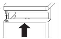
14. Slide the centre door bearing into the bottom left of the fridge compartment door and fasten to the housing.
